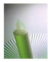
POLYVERSE is designed for clarification in Food & Beverage industries. The media is obtained by innovative materials with controlled and decreasing porosity, particularly pleated in order to allow the chemical regeneration of to performe an easier backwashing process. Materials of construction meet international guidelines for Food contact. Manufacturing is performed in a controlled environment.
